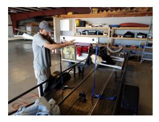
Place the fuselage cradle at the rear of the trailer. Elevate the trailer tongue. Place the wooden ramp at the end of the trailer. Roll, pull fuselage onto the cradle. Move the fuselage forward until the cradle engages the cradle latch. Make sure canopy is closed and latched. Install access cover on top of fuselage.
