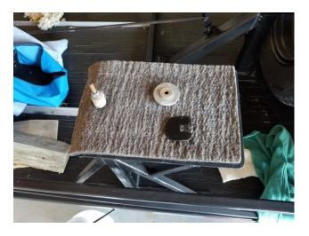
Place each wing on the trailer and install the washer and nut. Strap the wings down using the cuffs that go over the trailing edge.
