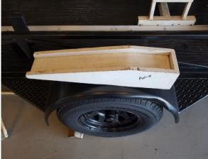
Adjust the fuselage position so the tail wheel sits in the recess in the floor. Strap the fuselage down.
