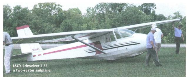
put into the air using several different techniques. LSC uses the aero-towing method. The sailplane is lifted into the air with the help of a tow plane (LSC uses a Scout 8GCBC), or tug, which pulls the small craft with a 200-foot rope. Once the plane reaches an altitude of 2-3,000 feet, the rope is released and the sailplane is free to ride the thermal currents that make up our atmosphere on an ideal gliding day.
